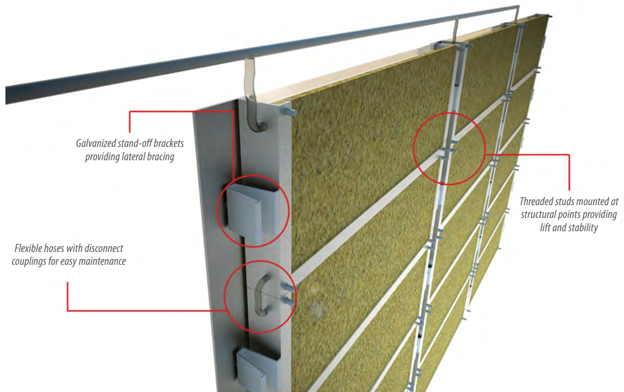
Figure 4.12.C - Thermal mass wall assembly diagram
