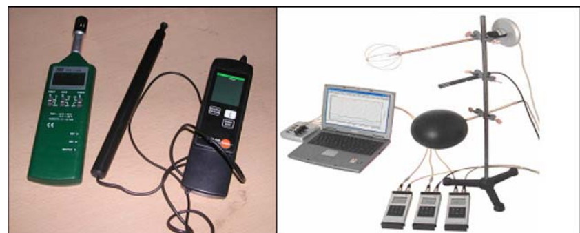
Humidity/Temperature Meter (TES1360) & hot-wire anemometer (Testo425)
